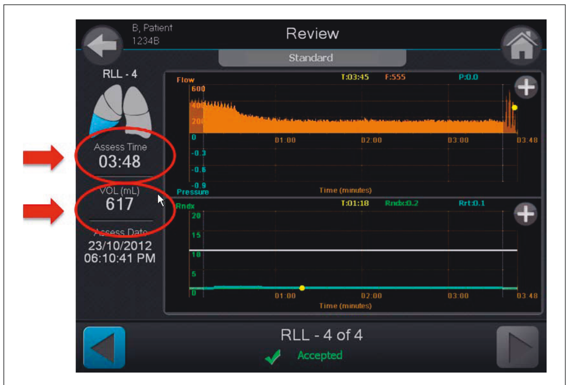
Fig. 5. Chartis system output screen demonstrating assessment time and volume of exhaled air from the target lobe during assessment. Example shows presence of collateral ventilation.
